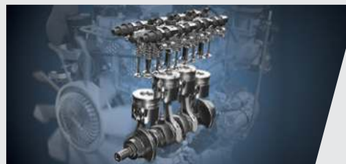
Diamond-like Carbon-coated Pistons and Injectors
